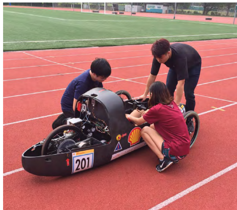
TP Eco Flash testing their energy-conserving, purge-free hydrogen car at Temasek Polytechnic. Images: TP Eco Flash.
