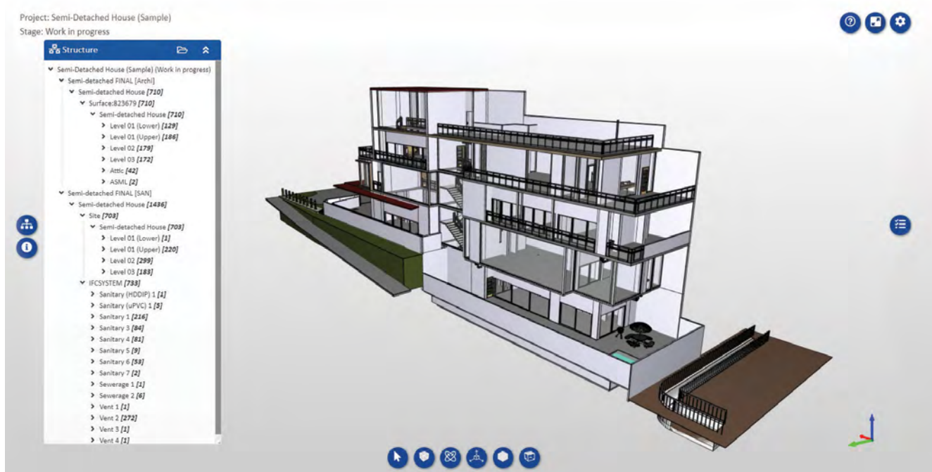
3D building models in IFC format can be viewed on the BIM e-Checker portal.
