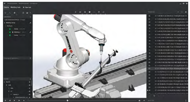
The new welding tools highlight how easy path creation in welding has become.
